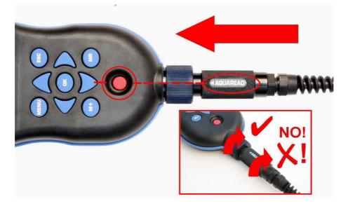
Always ensure the Aquameter<sup>®</sup> is switched off prior to connecting or disconnecting an Aquaprobe<sup>®</sup>. Align the **<Aquaread**<sup>®</sup> logo on the plug body with the red on/off switch on the Aquameter<sup>®</sup>, then press the plug into the socket and tighten the retaining collar.
