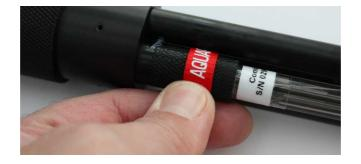
Slide the lanyard over the electrode and use it to grip the knurled body.
