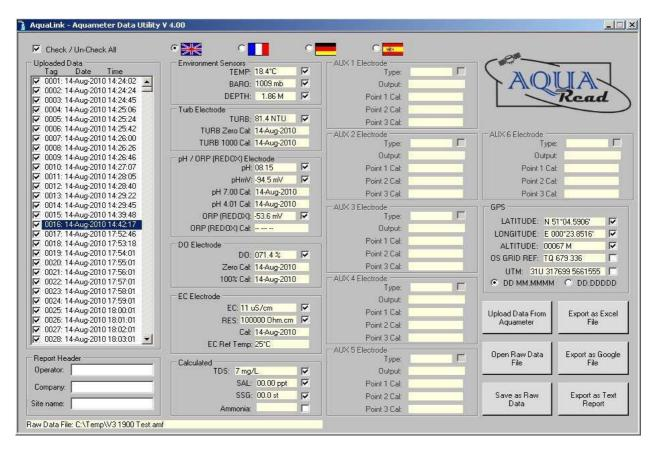
To view any of the logged data records, simply click on the desired Tag, date and time label as shown above. The data for the highlighted label will be displayed in the individual data boxes, which are grouped by electrode function. Any data that is unavailable or out of range will be displayed as dashes. To move up and down the Tag/date/time column, use either your mouse or the cursor up/down keys.
