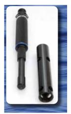
The AP-LITE is highly portable with its probe body measuring just 24mm in diameter and 250mm in length.
